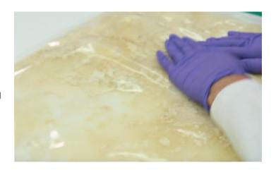
two at a time using the Thermo Scientific™ Dry-Bags Peristaltic Pump. Once filled, the Dry-Bags media bags are quarantined in the preparation room at least overnight and then, when needed, the trolley is wheeled to the laboratory where each Dry-Bags media bag can be connected to the dilutors.
